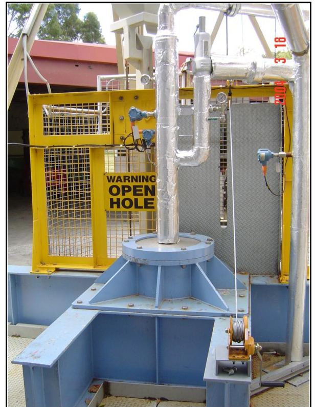
Figure 4: Exergen's pilot plant autoclave (4 tonne per hour).
