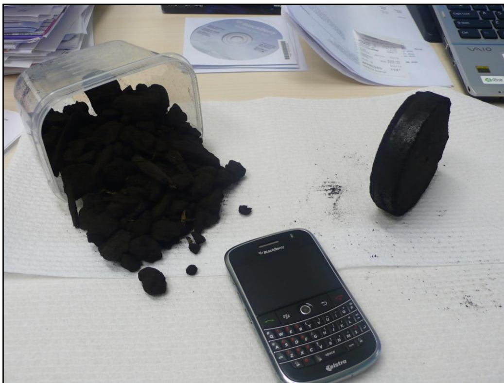
Figure 1: ROM coal (47% moisture) and resulting briquette (5% moisture).
