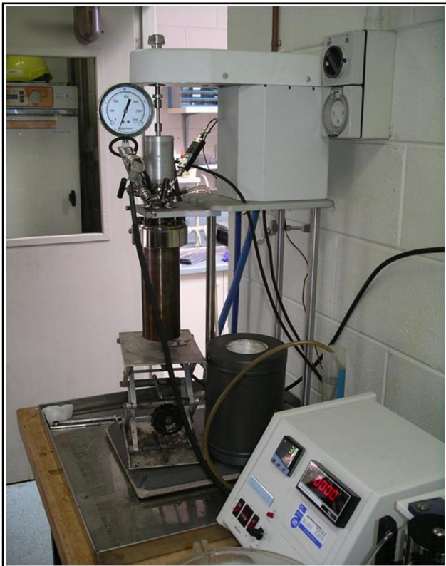
Figure 3: Exergen's laboratory scale autoclave (3 kilogram batch).
